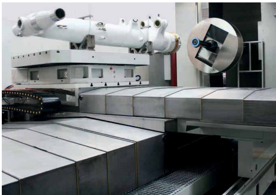
The AZ LBC range performs orbital grinding on the outer and inner diameters of heavy asymmetric landing gears on a rotating table, without moving the workpiece
