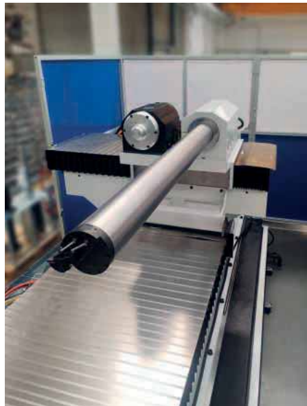
On GSB1900 the turning head is fixed on the grinding head carriage located beside the grinding electro-spindle
