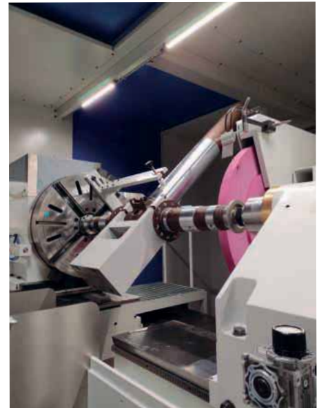
The AZ AKP range with gap bed allows external grinding of landing gears
