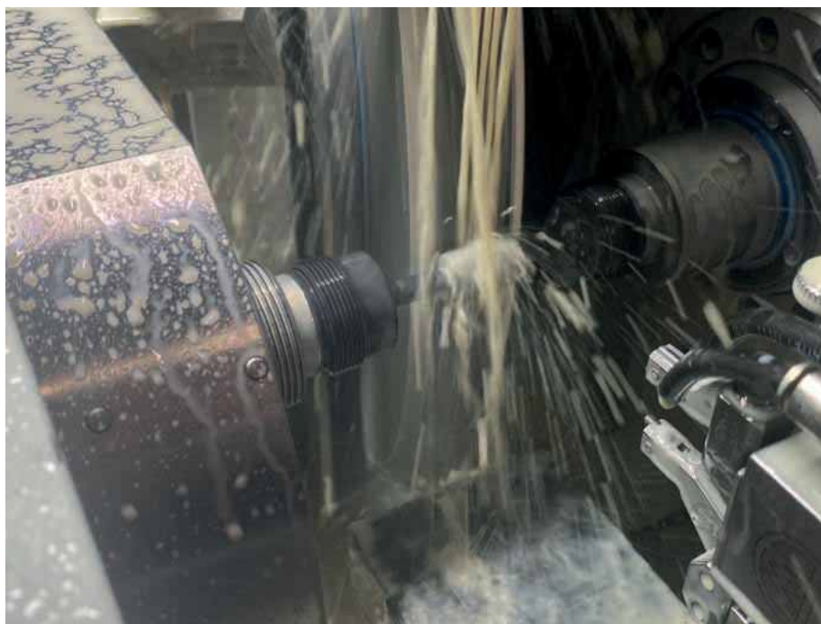
The K100 with a bearing between synchronised centre
