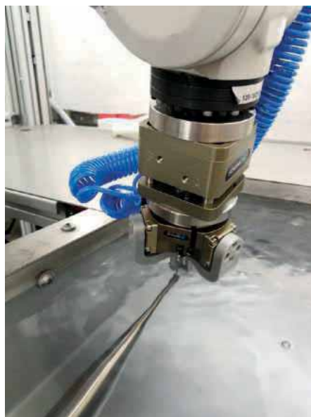
Ultrasonic deburring takes place in a water basin in which components are advanced to the high-frequency ultrasonic sonotrode.
