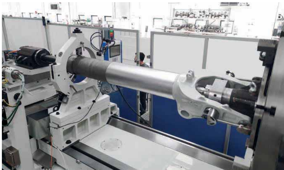
The GSB1900 grinding machine combines both internal grinding and turning operations for heavy asymmetric landing gears in a single machine solution
