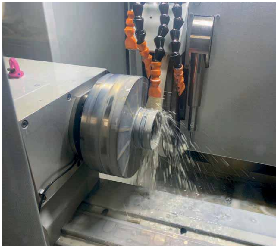
The Kellenberger K10 with a magnetic chuck grinding Gamet Bearing
