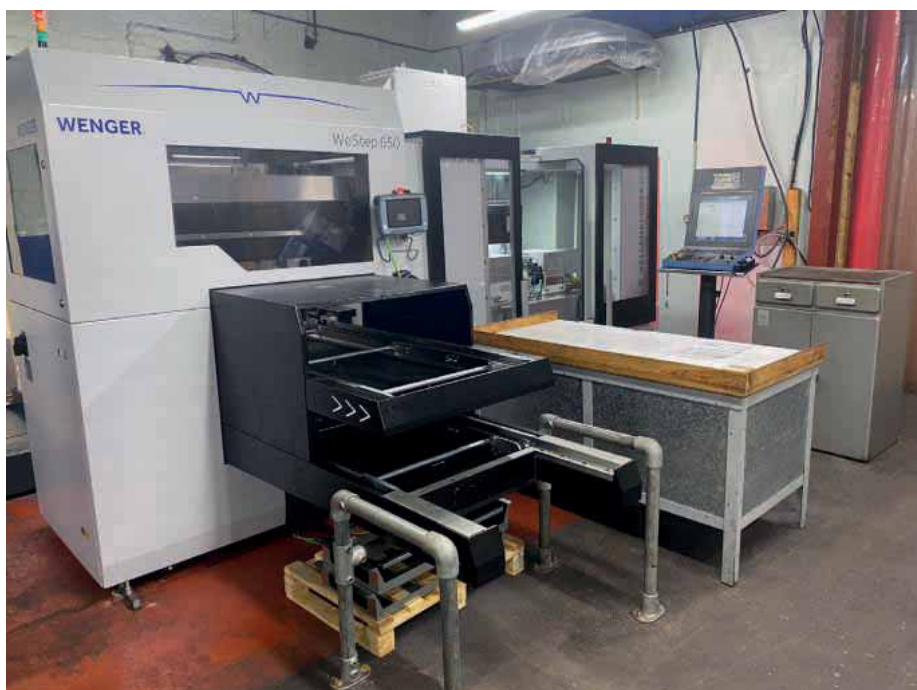
Wenger Weststep automation system feeding the Kellenberger
