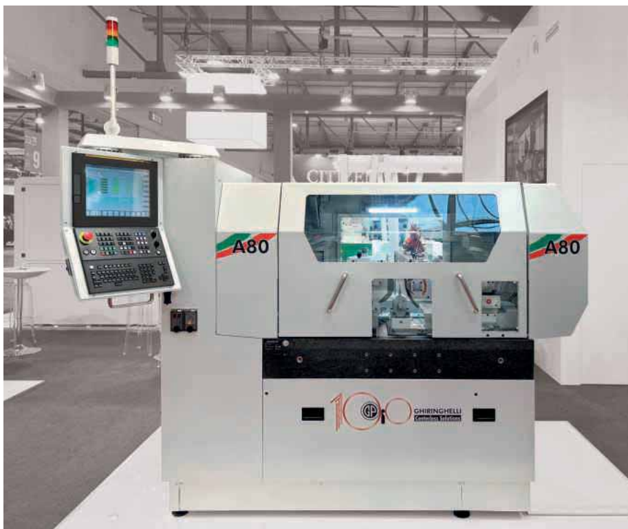
The Ghiringhelli's A80 centreless grinding machine with fixed centre is equipped with the new CNC FANUC Oi-F Plus
