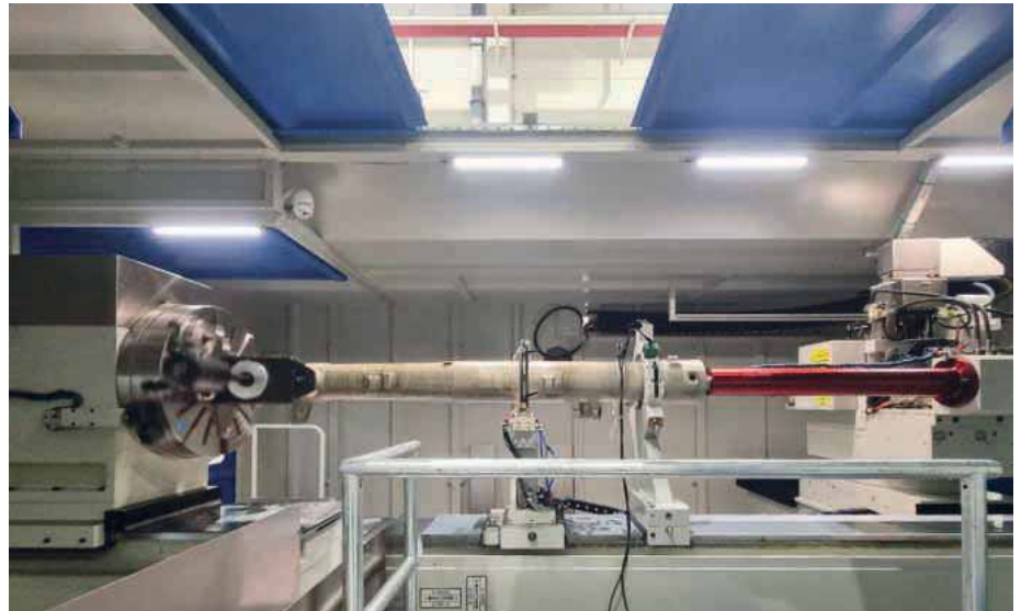
The internal grinding of deep holes on landing gears is carried out using special electro-spindles equipped with various interchangeable extensions
