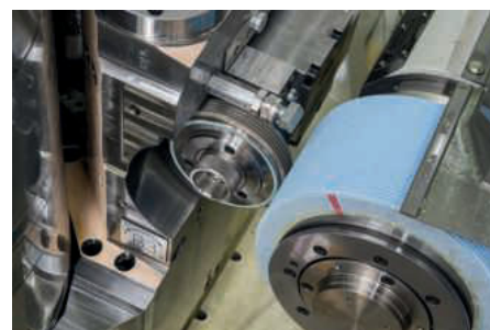
Multi-rib dressing of a vitrified grinding worm
