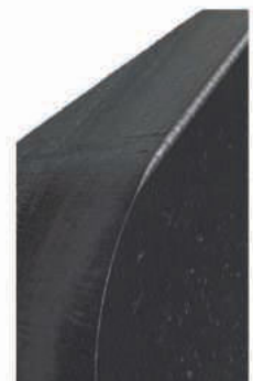
Example: Transition from a large edge to a 1 \mu\text{m} edge
