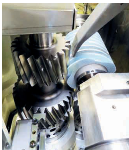
Generating grinding of a gear with interfering geometry
