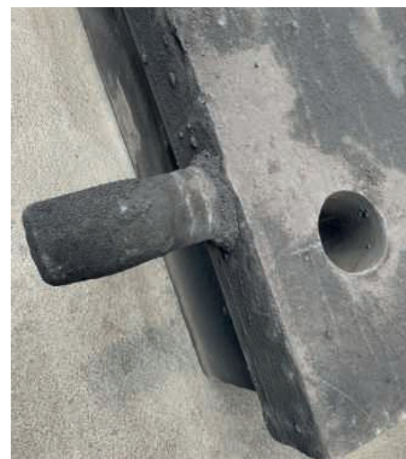
The aim of the blasting is to remove sand from the workpieces
