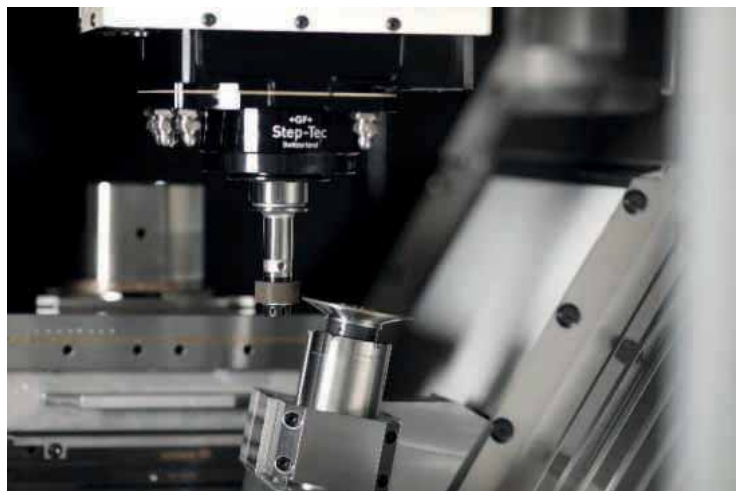
Inclinable and adjustable dressing spindle close to the working area for a fast grinding setup and process
