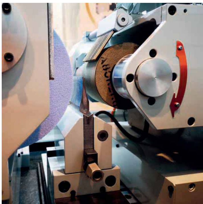
The new Ghiringhelli A80 centreless grinding machine with fixed centre has perfect technical features for very small parts
