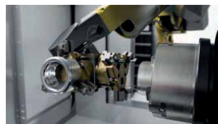
Loading and unloading situation with STUDER roboLoad
