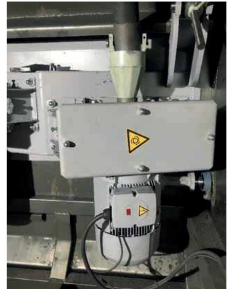
A glance at one of the two horizontally mounted AGTOS high-performance turbines
