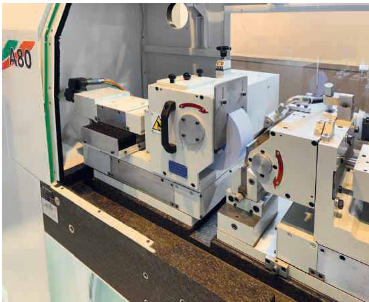
The new A80 centreless grinding machine with fixed centre is conceived with six CNC axes on a natural granite machine bed
