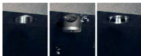
Mechanical deburring solutions with moving blades, such as the COFA tool from HEULE shown here, deliver finished and deburred workpieces directly from the machine
