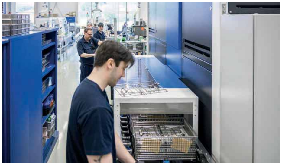
The system concept as well as numerous features available as standard options, such as the three flood tanks for the wash, rinse/rinse or preserve process steps, were major decision criteria in favour of the EcoCcompact
