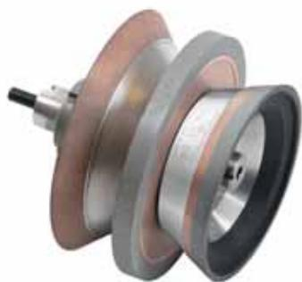
The support rim of the new Cafro E-Cup 11V9 wears at the same rate as the abrasive rim so operators no longer have to stop the machine and disassemble the wheel to relieve the body, saving time and increasing total productivity.
