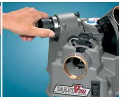
detracting from the tool's performance. One side is ground away and then the other to split the point, with both motions reaching a predetermined stop each time. Two extra cutting edges are added, reducing by up to 50 percent the down force required for machining.
