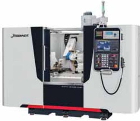
*JAINNHER JHPA-2003CNC Plunge Cylindrical Grinding Machine.*
