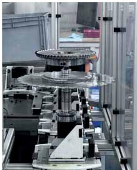
*TCT Saw blades on the QXD250 and HC4 chain magazine automation system.*
