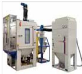
The compact Guyson RXS400 (Rotary Indexing Spindle) blast machine delivers an accurate, consistent and uniform quality of surface finish, coupled with high productivity.
