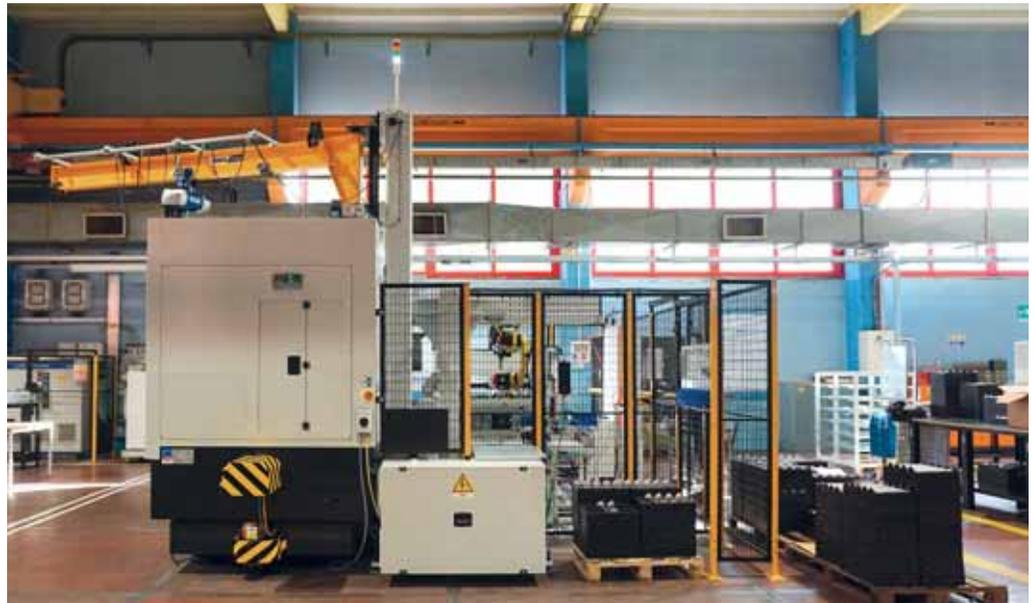
*The solution provided was configured as a robotic isle and the automatic feeding loaders are handled by a FANUC anthropomorphic robot.*
