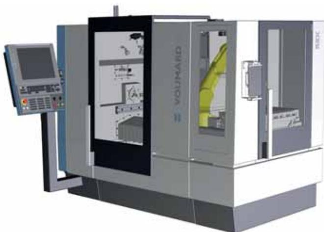
*Compact machine, compact automation. The footprint of the of the VOUMARD 30 with robot cell is just 2.30 x 1.80 m.*
