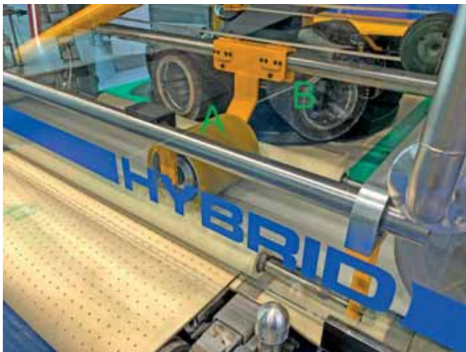
2 Oscillating methods – starting with the sanding belt (A) and ending with the gear head (B)
