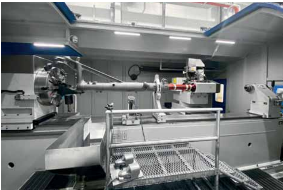
The internal grinding of deep holes on the landing gear is carried out using special electrospindles equipped with various interchangeable extensions.
