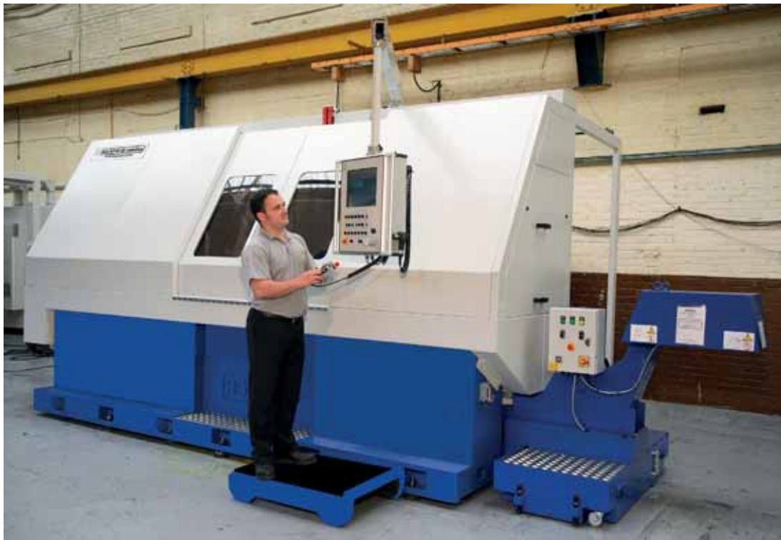
Built to last: an original Holroyd 2E-volution CNC rotor milling machine, pictured when new.
