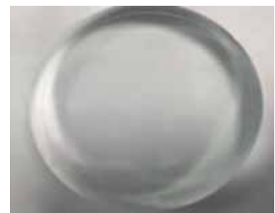
Lapped and polished quartz.
