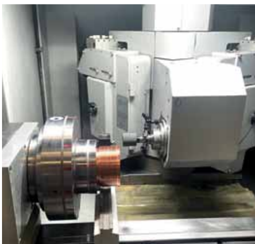
Internal grinding of a workpiece with problematic material combination.
