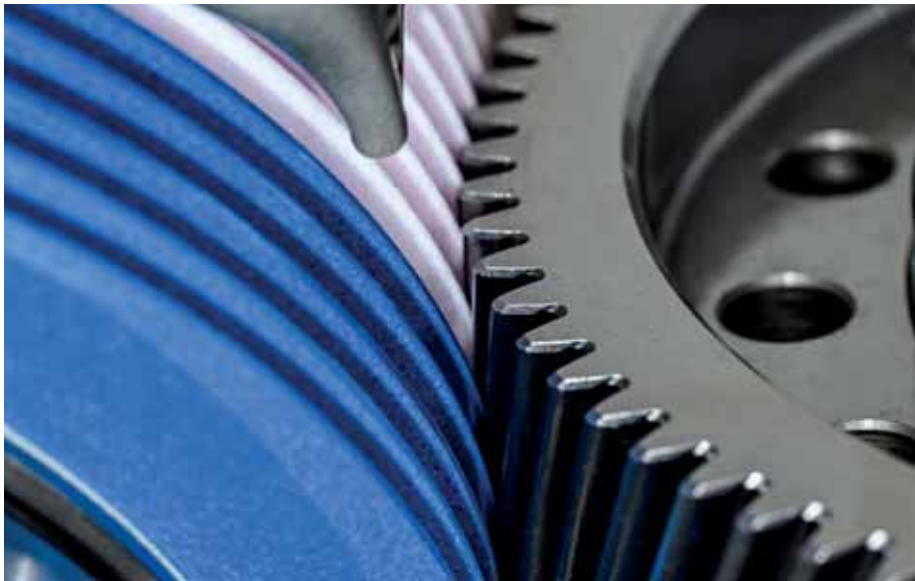
Figure 1 - Grinding worm for the polish grinding of gears.
