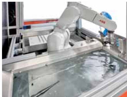
The robot loading station on the ultraTEC A25 from Vollmer.
