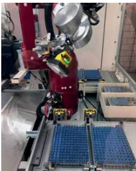
Mass deburring of parts on an MF machine for the automotive sector.
