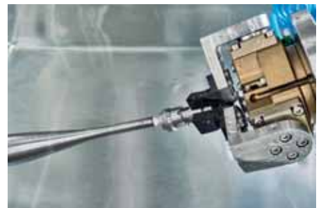
The ultrasonic horn and parts gripped in the ultraTEC A25 machine from Vollmer UK.
