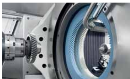
Gleason Combi Honing with two honing tools in one setup, seen here as a polishing application.
