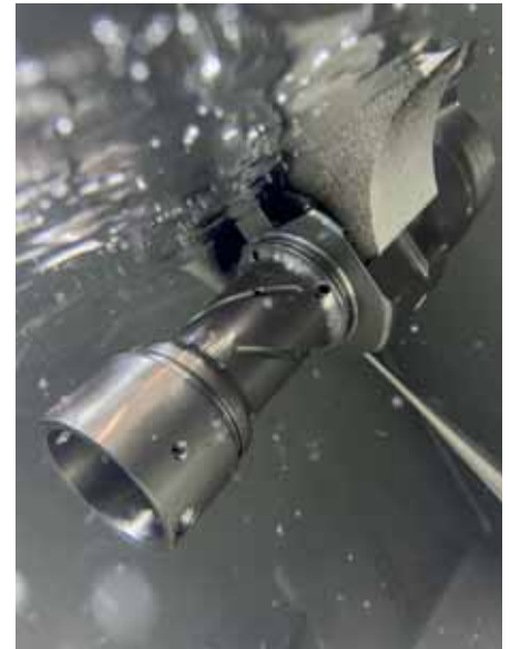
The process of ultrasonic deburring of the hydraulic blocks uses ultraTEC technology with an ultrasonic sonotrode.
