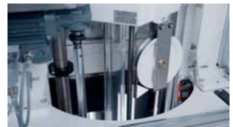
2-station swivel table, including honing fixture and safety enclosure.
