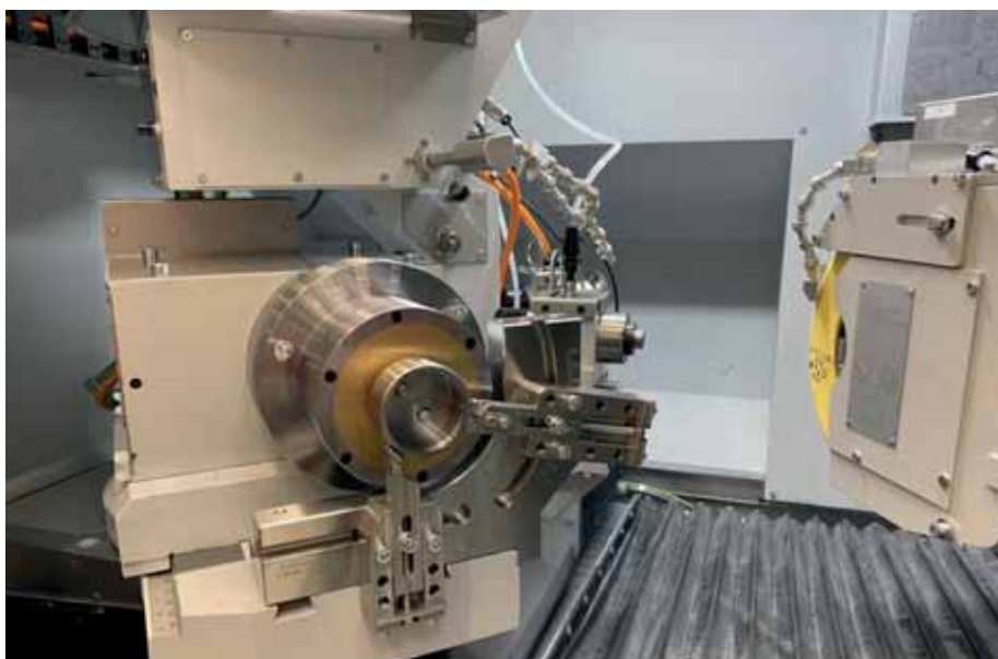
Exemplary clamping device for bearing production: magnetic chuck and support shoe device.
