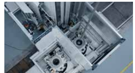
2-station swivel table, including honing fixture and safety enclosure.
