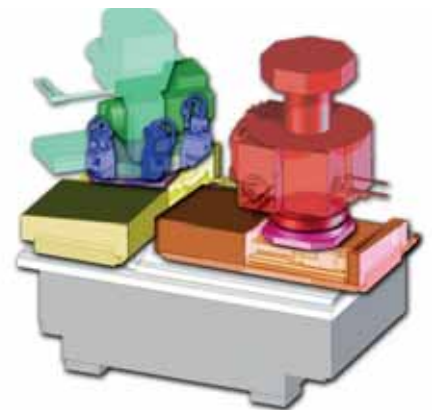
Unique machine concept: The patented B2 axis with table turret of the VOUMARD 1000.
