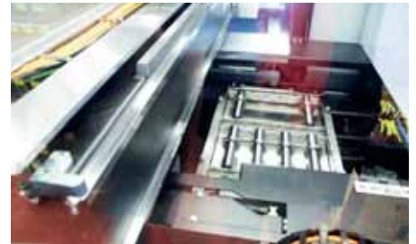
Interior of the WeFlex loader with line gantry and pallet changer.
