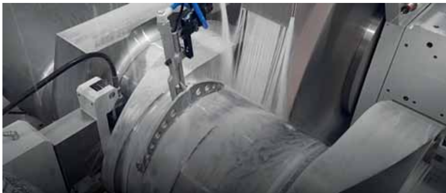
The Marposs diameter measurement system with part tracking ensures greater precision and reliability.
