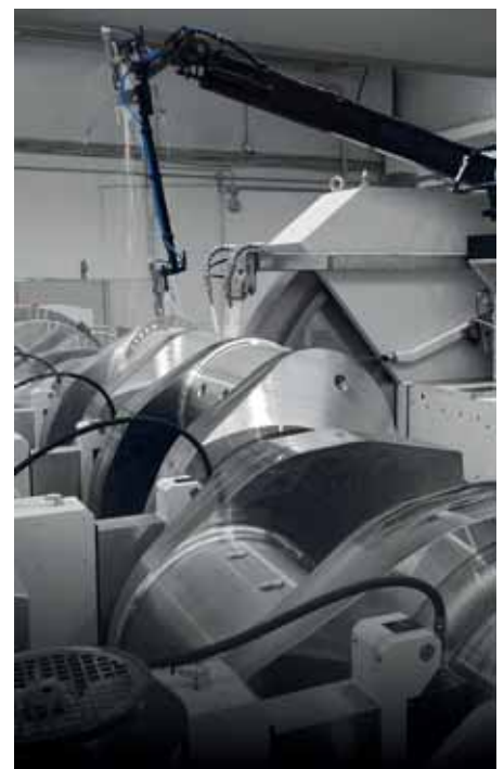
The AZ orbital movement for pin chasing is equipped with a B axis for taper correction.
