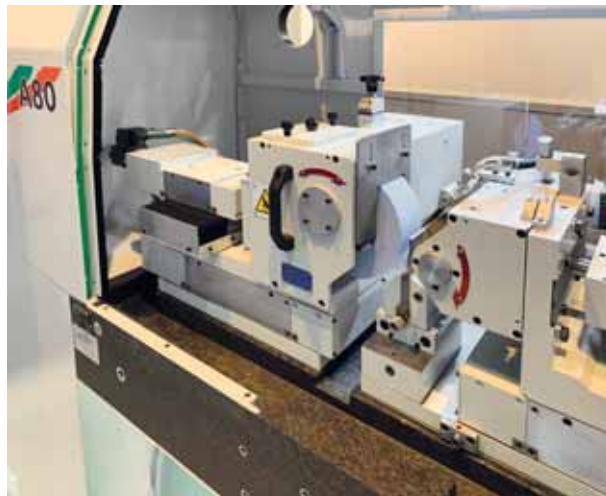
The A80 centreless grinding machine has six CNC-controlled axes and a natural granite bed.
