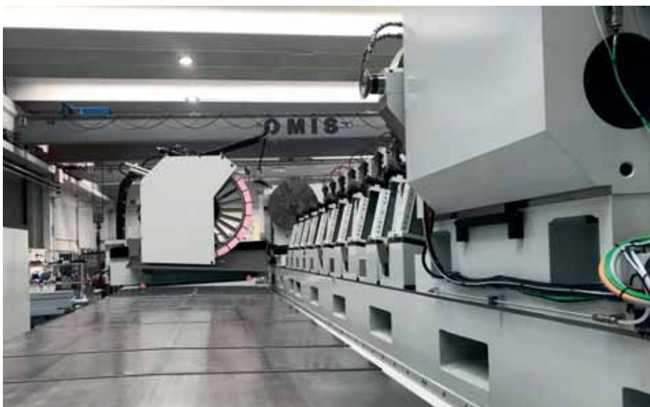
On DB12500 the wheelhead moves on a hydrostatic carriage powered by a linear motor on hydrostatic guideway.
