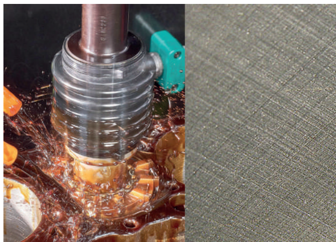
A honing tool applies engineered abrasives to create the distinctive crosshatch pattern that improves oil retention and reduces stress in internal combustion engine bores.
