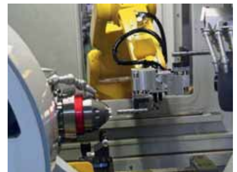
Headed punch being loaded head-first into the GDS Shark chuck on the MX7 – the head is accommodated inside the chuck while the shank is ground.
