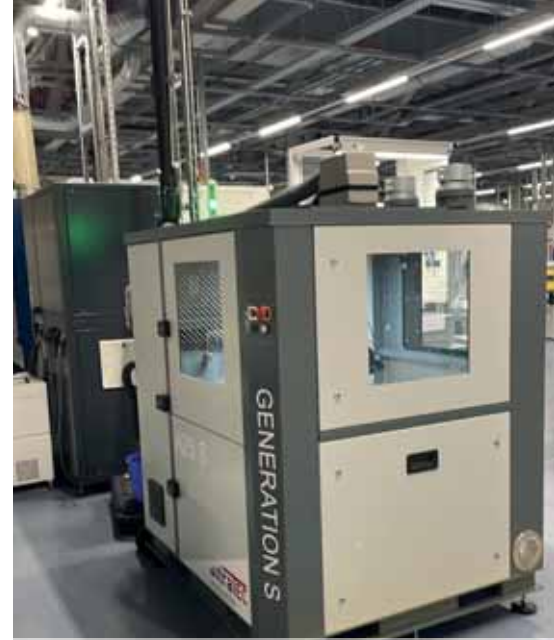
With the ultraTEC A25 S ultrasonic deburring system, Aesculap can deburr its bone saw blades contact-free and automatically.
