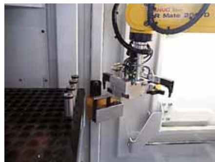
Custom flip station on the ANCA Robomate: headed punches are rotated and oriented for reliable, fully automated loading into the MX7.
