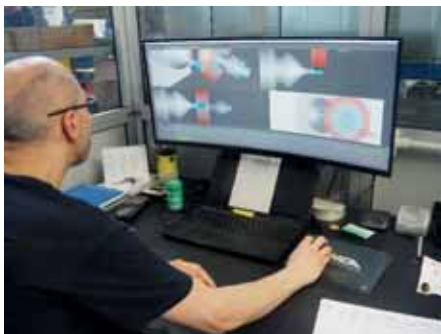
Technical engineer Claudio Innamorati using ANCA's CIM3D software to simulate and verify punch grinding processes before production.
