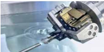
During ultrasonic deburring, an industrial robot guides the components in a defined position.
