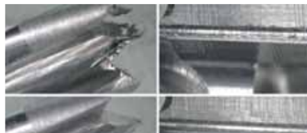
Before and after - Selective ultrasonic deburring with the ultraTEC A25 S removes unwanted burrs.
