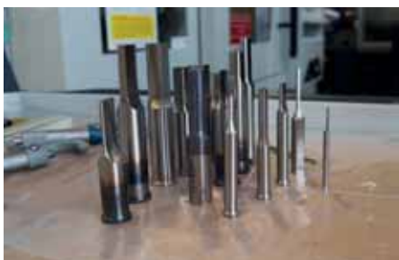
Selection of steel and carbide punches manufactured by Nuova Ret for high-speed stamping, thin blanking, deep drawing and perforating applications.
