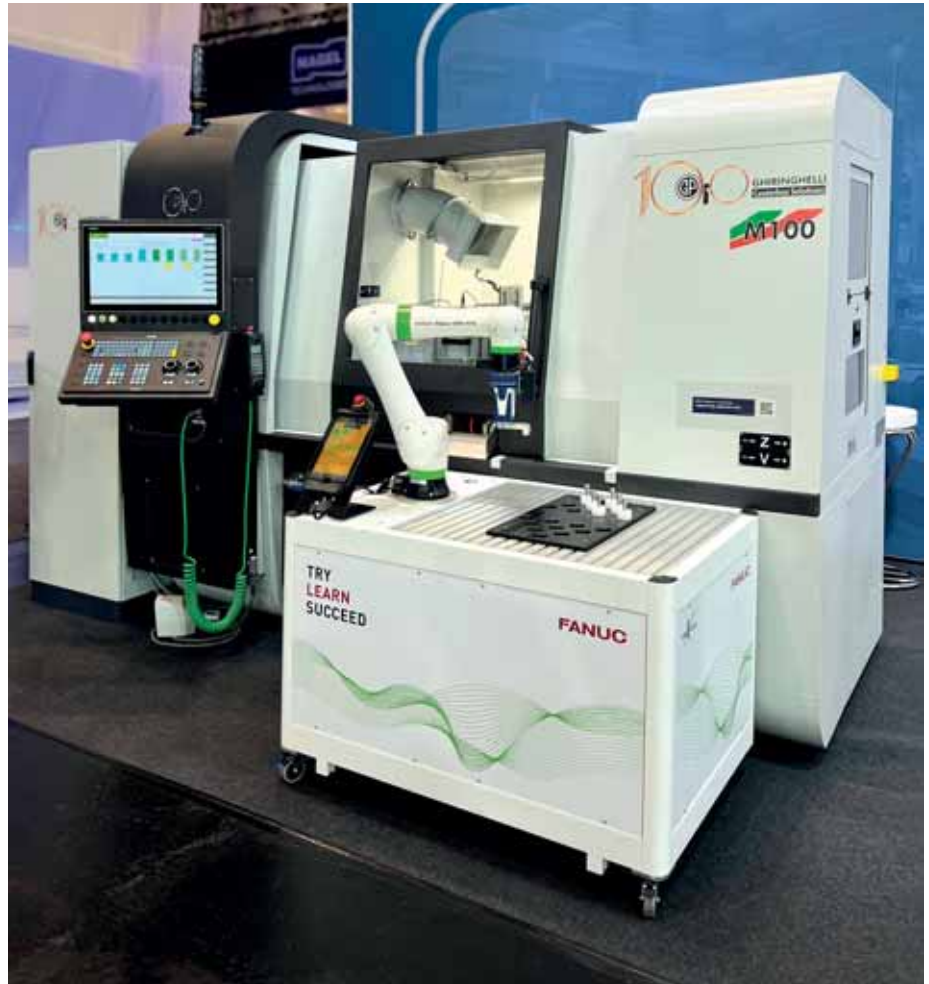
The M100 integrates automatic machine feeding systems such as the FANUC CRX-5iA cobot.
