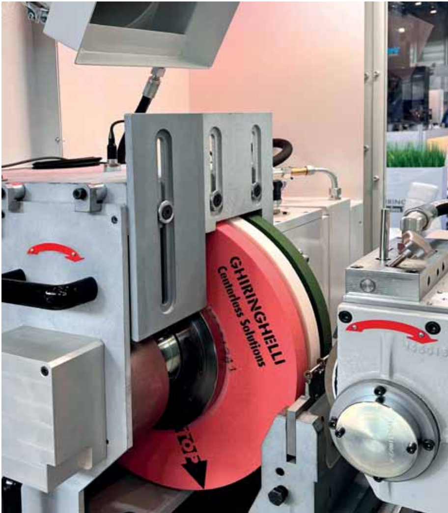
The M100 centreless grinding machine grinds components with diameters between 0.50 and 20 mm, lengths up to 135 mm, with the utmost accuracy.
