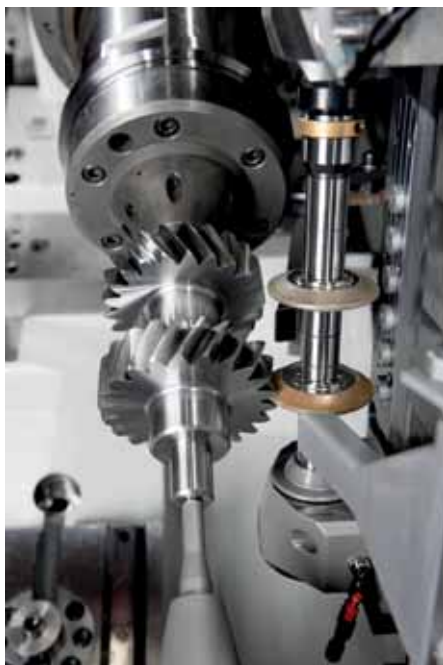
Several grinding wheels can be used simultaneously on the grinding spindles of the VX machines.
