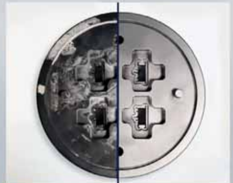
Extrusion Die BEFORE vs AFTER Processed using our automated radial arm solution
