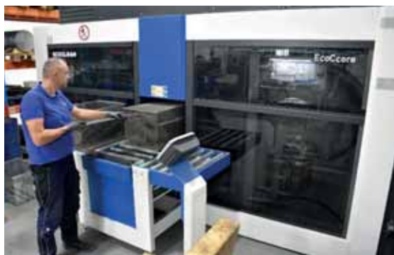
The parts are cleaned prior to heat treatment to remove contaminants and emulsions in a compact EcoCcore solvent cleaning system from Ecoclean, sourced through MAP PAMMINGER.
