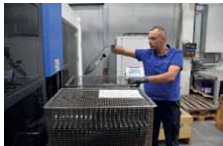
Cleaning is carried out in 670 x 480 x 400 mm baskets from the manufacturer Kögel with lids and spring-loaded compartment rods to separate the parts.
