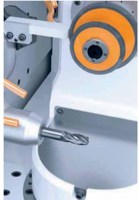
The new optional roughing unit for the Vgrind 360 enables automatic opening of the abrasive coating during production
