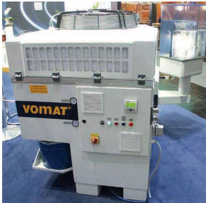
While in full-flow filtration, VOMAT filtration systems permanently provide clean oil in NAS 7 quality. On-demand filtration and back-flushing reduce stress on filter and machine components while reducing energy consumption
