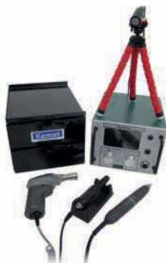
With state-of-the-art ultrasonic technology, the unit provides automatically adjusted frequency up to 45 watts output with 30,000 stokes per second, and variable stroke length between 3 and 40 µm. A brushless micromotor provides up to 300 watts of power with three speed ranges: 1,000-15,000, 15,000-30,000, 30,000-50,000 rpm and reversible rotation of the 2.35 mm diameter collets. Last but
