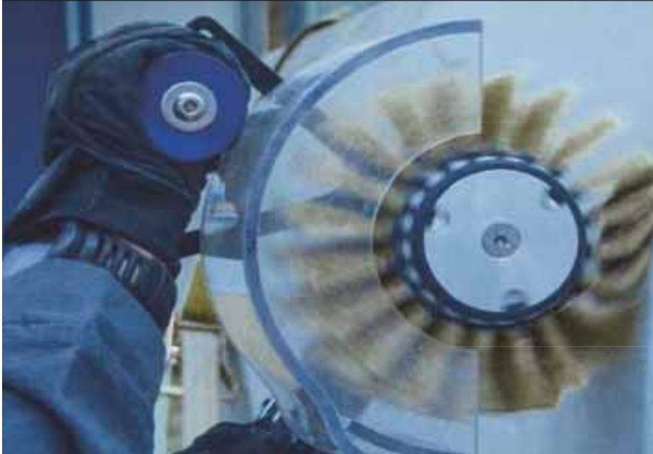
TYROLIT POWER offers a new, innovative shape for machining extremely hard coatings and surfaces. A combination of natural-hair brushes and a layer of net backing with diamonds enables a controlled surface finish in the shortest time. Use TYROLIT POWER instead of conventional dual action sanders or abrasive cloth flaps and significantly reduce your costs and machining times
