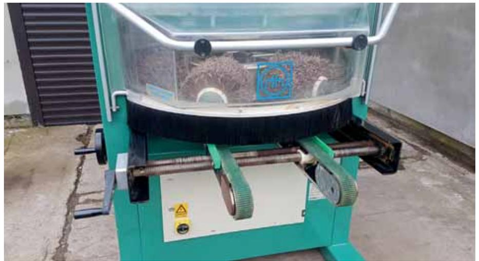
developed and the first automatic feedthrough machine for denibbing of, for example, kitchen cabinet doors was presented at the LIGNA exhibition in Germany:
