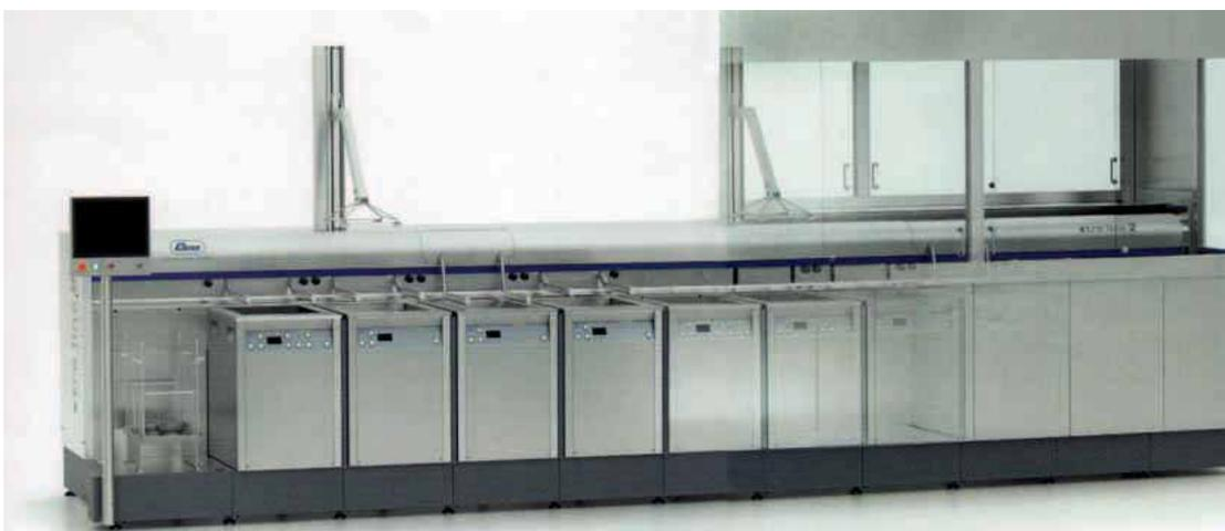
Available in a variety of sizes, they feature a welded stainless-steel tank, double lid with thermal and acoustic insulation, thermostatically controlled indirect heating in the side walls, and an electronic control with digital time/temperature display. A level guard cuts off the heating and ultrasonics if there is insufficient liquid in the tank.
