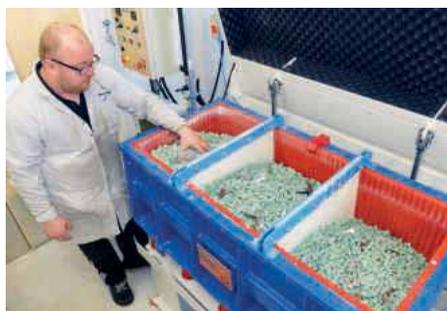
chemical blacking or painting. Nine out of 10 people bring in sample components to be finished on a free trial basis, so they can see the process in action and its effectiveness. Many parameters are taken into account, including the number of parts to be finished per batch, frequency of production, drainage and noise issues, the size of components and how vulnerable they are to impingement damage.
