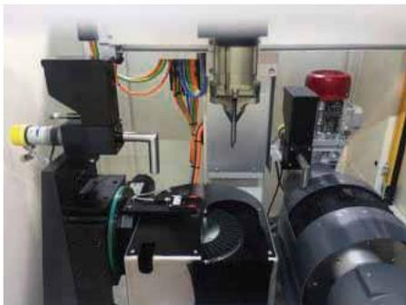
Magnetfinish machine for cutting tools
