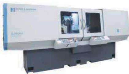
Although the machine at MACH has a 1,000 mm grinding capacity, a longer 1,500 mm capacity version is available. The Suprema model has a universal wheel head with two external wheels and one internal.
