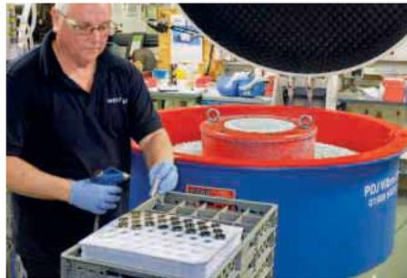
parts machined to extremely tight tolerances are suitable candidates for vibro finishing. As the latter may not be generally appreciated, a number of case studies will be cited where PDJ Vibro equipment is being used to automate the finishing of very high precision components, without surface damage or dimensional change.
