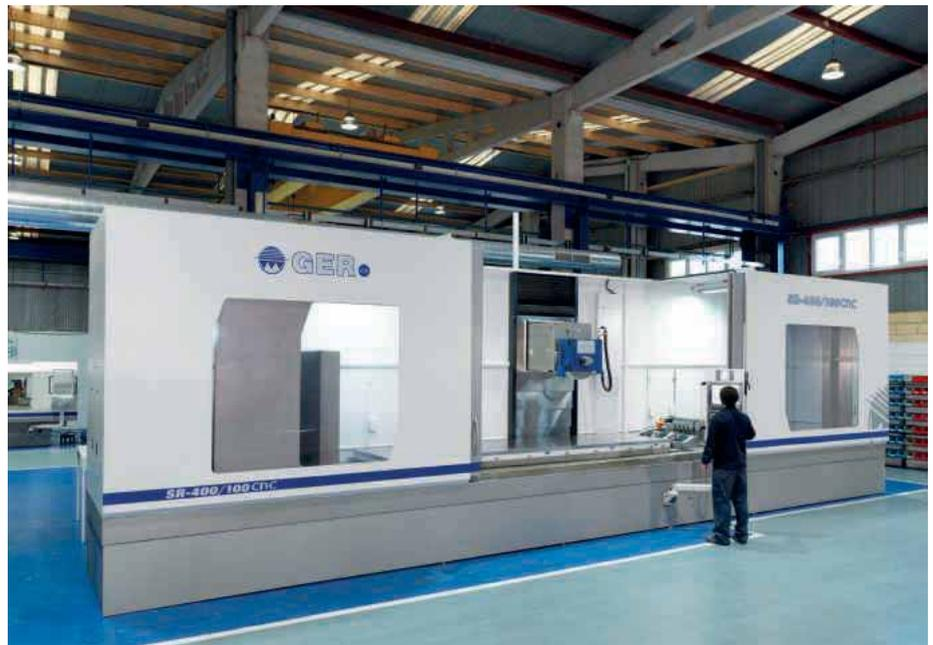
slideways incorporate precision ball screws, FANUC drive motors and Heidenhain linear scale feedback.
