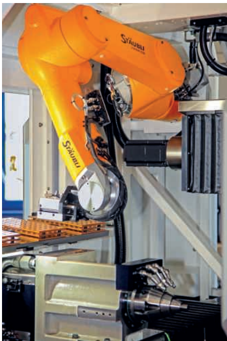
A Stäubli robot arm automates loading and unloading of blanks and tools into and out of a hydraulic expansion chuck (bottom right) in a Strausak U-Grind tool manufacturing and reshaping machine
