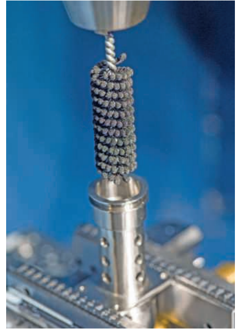
New BRM flexible hones are simplifying the task by incorporating one of the toughest, hardest materials on the planet - Cubic Boron Nitride (CBN)
