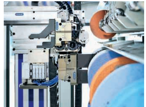
Two powerful SCHUNK universal grippers PGN-plus safely assume the handling of the tools
