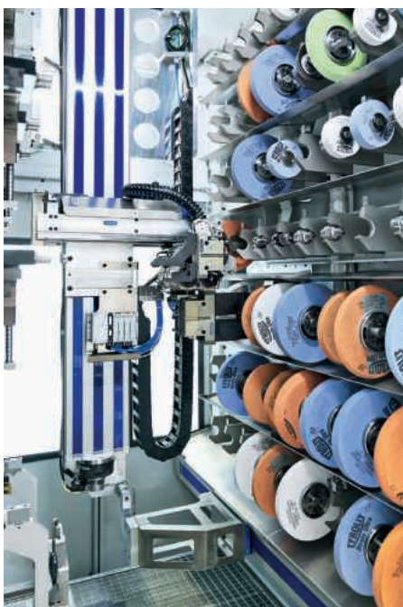
The SCHUNK axis system facilitates highly flexible unmanned grinding operations
