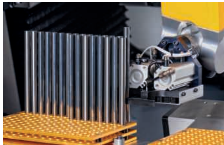
To extract a carbide blank from a tightly packed pallet, in this case with 150 positions for tools of 10 mm diameter, the robot arm has to be moved with high accuracy in all six axes simultaneously
