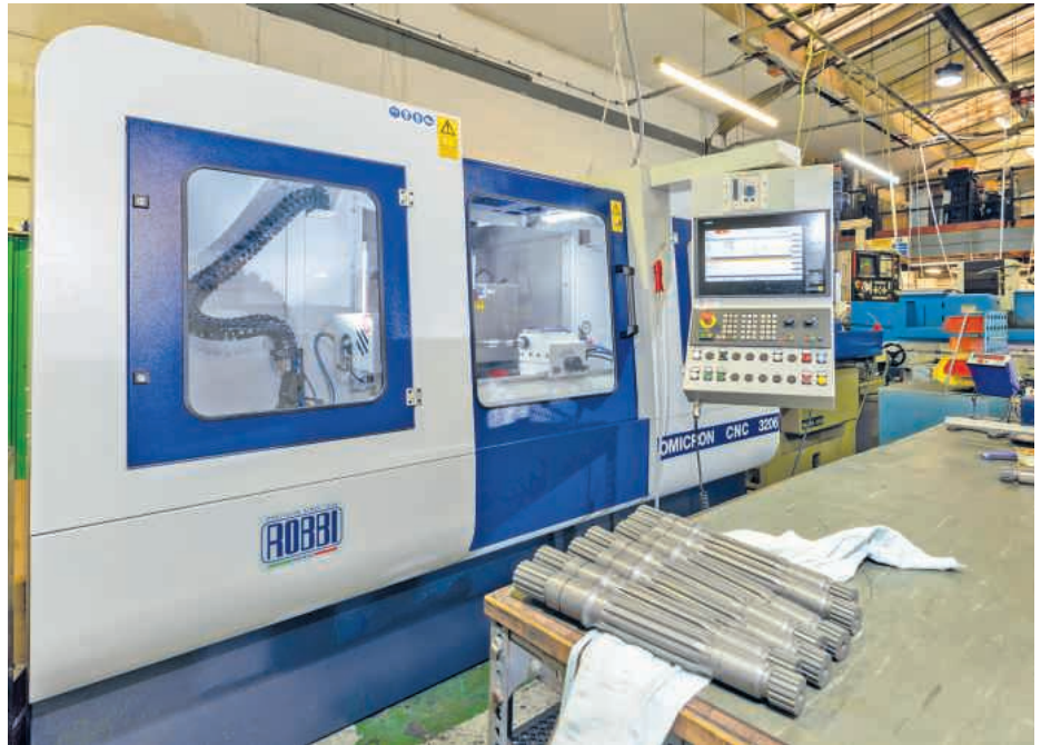
The Robbi Omicron CNC3206 CNC Universal Grinder from RK International Machine Tools is giving Muffett Gears added flexibility and capacity as it expands export sales to China
