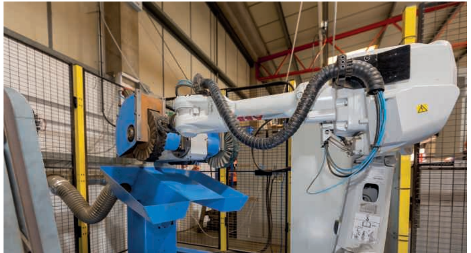
The Autopulit robot grinding, finishing, polishing and graining cell, with pallet loading and component sensing systems installed at Focus SB by Ellesco
