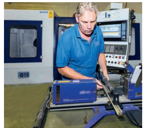
Shift Leader Rob Hudson checks the ground parts using a laser micrometer
