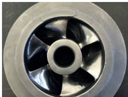
By machining an impeller for a pump manufacturer, the efficiency could be improved by 15 to 20 percent
