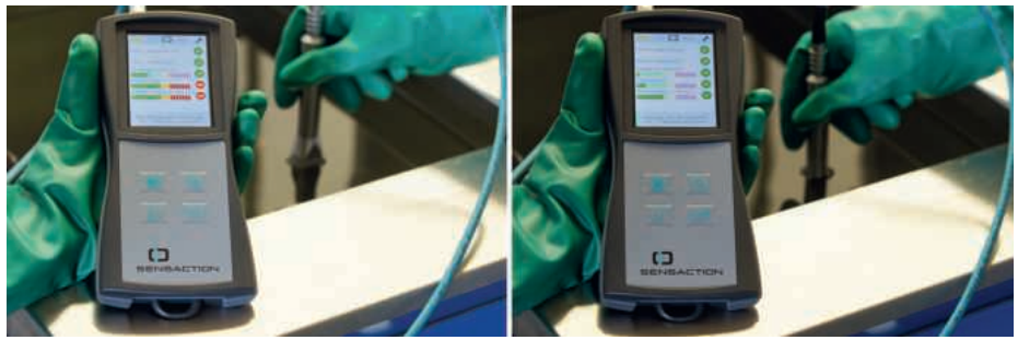
With aqueous media, the concentration of cleaning agent can easily be monitored inline or, as here, with a mobile device (photo SensAction AG)
