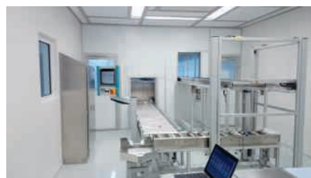
Here the cleaned parts are discharged into the clean room via a material air lock after passing through a fully enclosed cleaning line equipped with its own supply of purified air (photo EcoClean)
