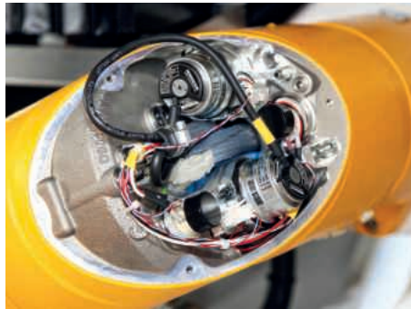
Inductive HEIDENHAIN EQI 1100 rotary encoders measure the position of each of the six robot axes
