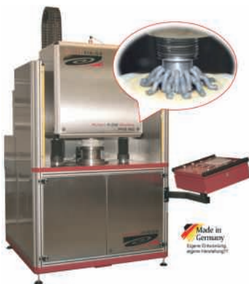
By machining an impeller for a pump manufacturer, the efficiency could be improved by 15 to 20 percent
