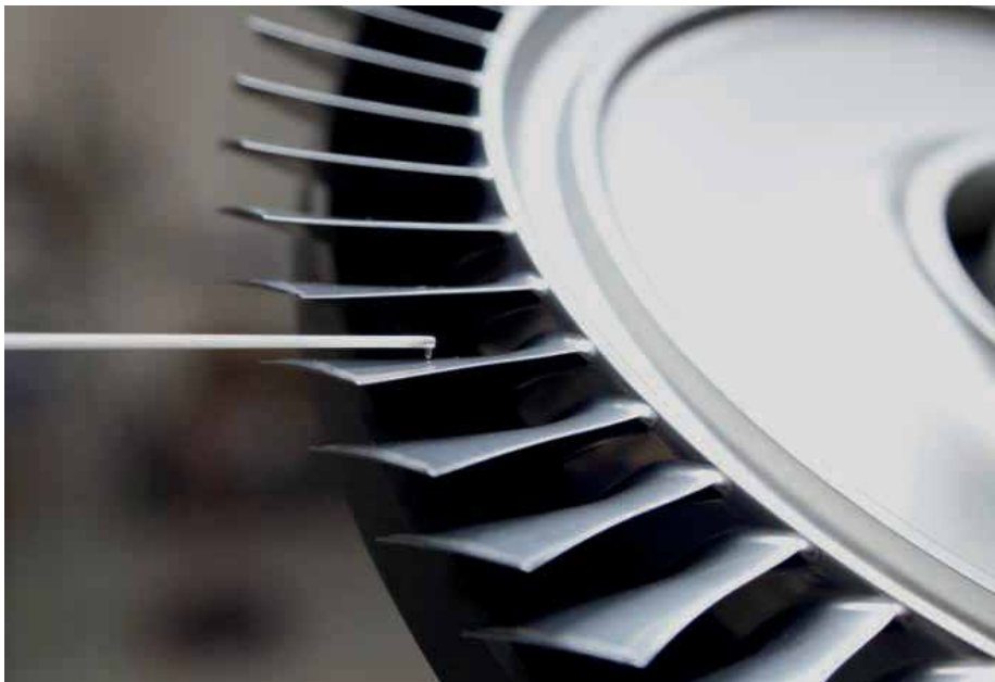
Long with smooth airflow surfaces, blisk performance greatly depends on a precise and uniform blade profile, especially along the leading and trailing edges
