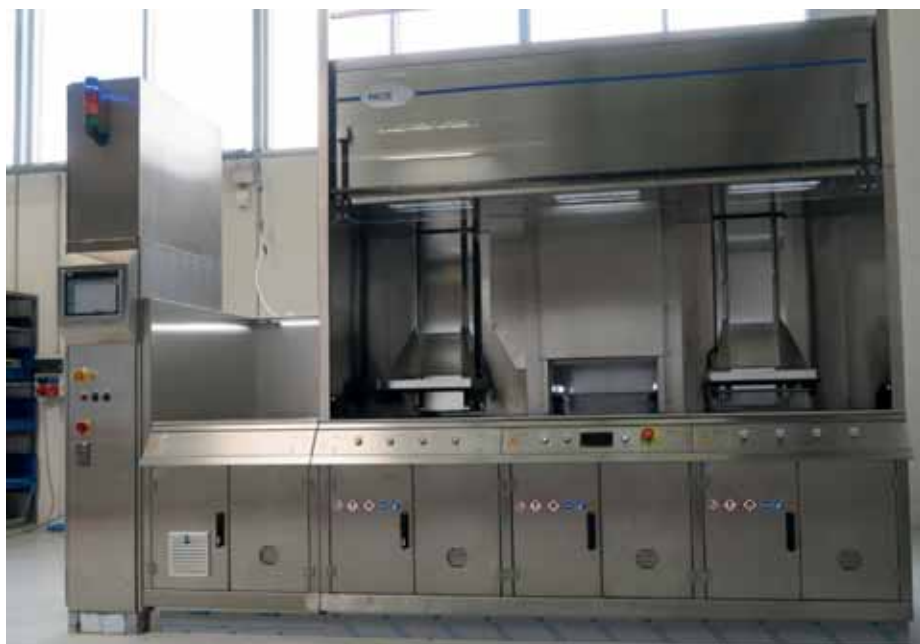
The facility for cleaning the goods carriers is equipped with two cleaning stations and one drying station and is integrated in a cleanroom
