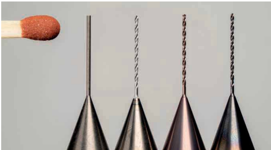
The evolution of a carbide drill bit on the Laser Line Ultra, from left: 0.5 mm diameter carbide blank, 0.45 mm diameter drill after laser processing and the drill after TiAlN then AlTiN coating
