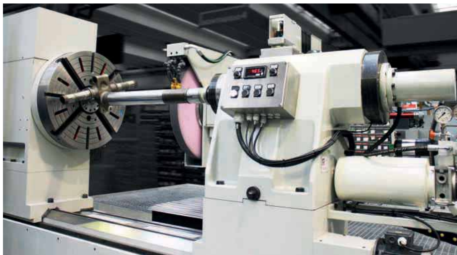
The tailstock has hydraulic constant pressure controlled by load cell
