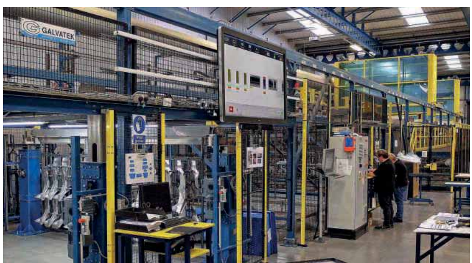
A Galvatek automated anodising line supplied by Turbex to BCW Treatments, Burnley
