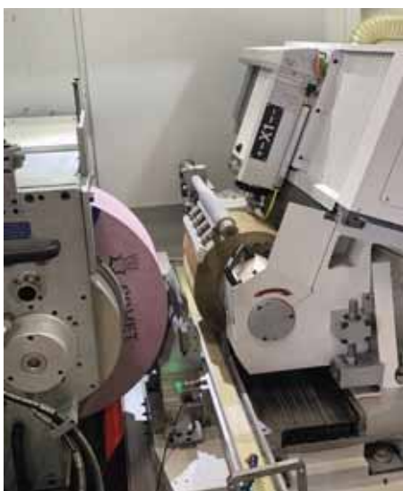
The grinding wheel mount head has wheels with Ø 610 mm x L 250 mm and the control wheel mount head has wheels of Ø 305 mm x L 250 mm
