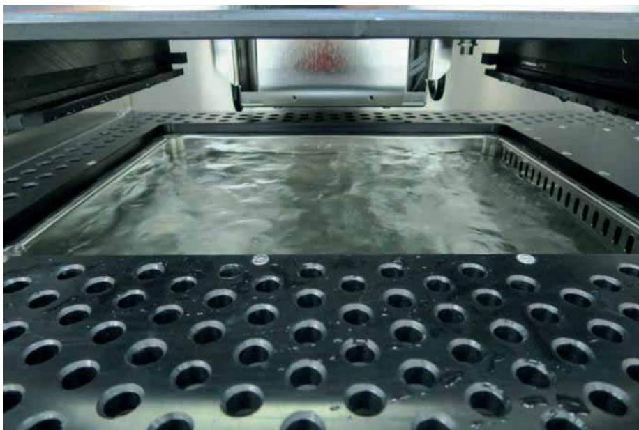
Forty-eight vibrating elements are installed on the floor of each of the cleaning tanks. They reliably deliver the required high output of 2,400 watts (Photos courtesy of Weber Ultrasonics AG)
