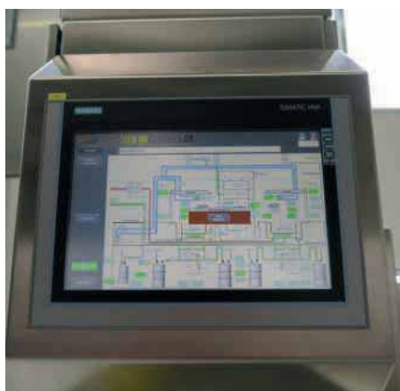
The ultrasonic technology is managed via the Profinet interface integrated in the generator in the HMI for the complete system
