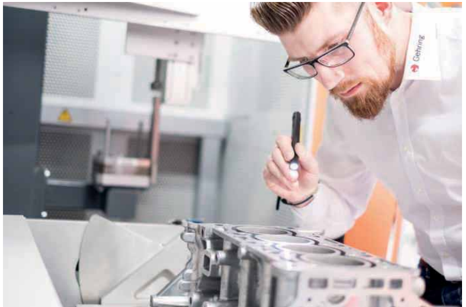
Nanohoning is used to produce engines with coated cylinder liners, which makes them more compact and efficient. Gehring supplies corresponding equipment to car manufacturers worldwide
