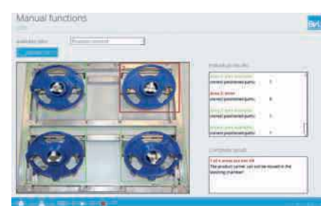
Libelle Product Control uses the "Position Monitoring" app to detect incorrectly positioned components on the workpiece holder
