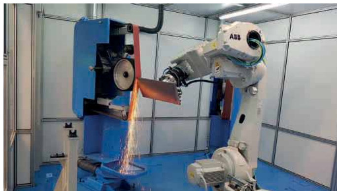
Autopulit weld dressing robot cells offer major productivity gains
