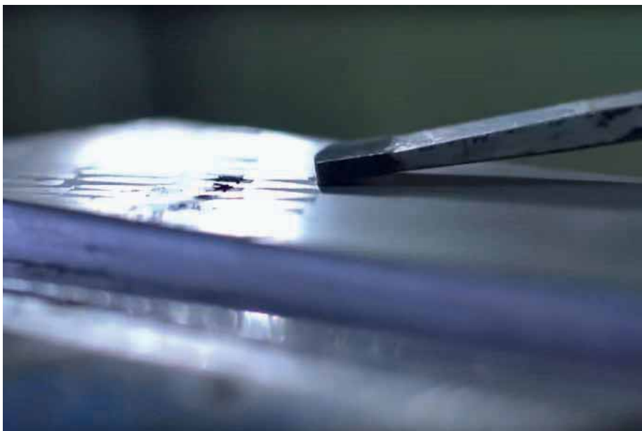
Hand scraping, as it is used by Okuma, is extremely time-consuming and requires a lot of experience and skill
