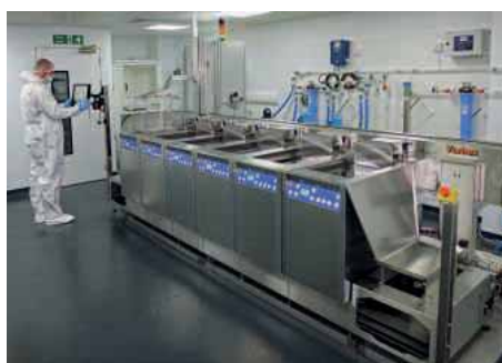
A Turbex Pro 550 six-stage, aqueous, ultrasonic cleaning line installed at Assembly Techniques, Dukinfield
