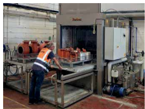
A Turbex AC-1.7-2 aqueous cleaning machine for batch processing cast iron components supplied by Turbex to Selwood's pump production facility in Hampshire
