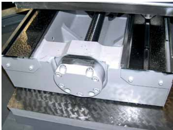
Okuma grinders possess hand-scraped sliding surfaces that help to achieve extreme precision and longevity
