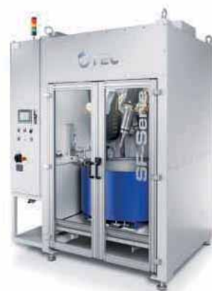
The SF4 stream finishing machine from OTEC is capable of smoothing individual turbine blade surfaces to values of R_a < 0.2 \mu m in minutes
