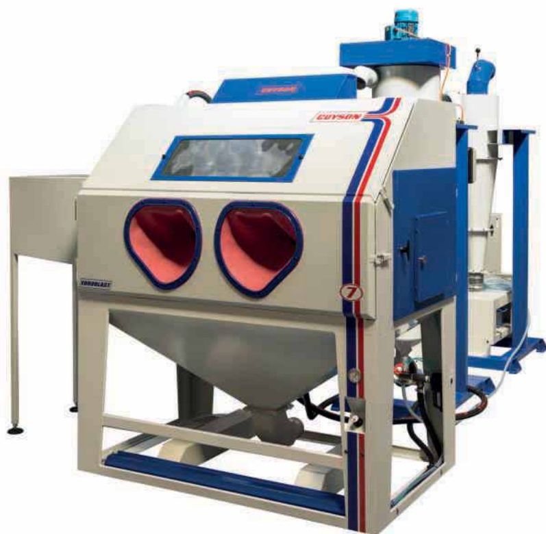
The Guyson Euroblast 7PF blast cabinet with extension box and high efficiency cyclone
