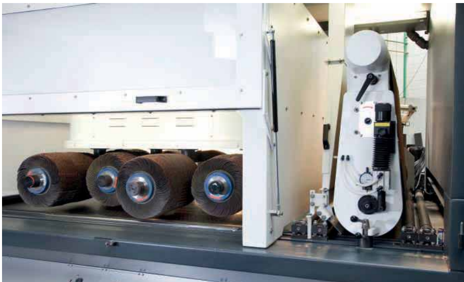
The combination of abrasive belt and rotary brushes on Timesavers machines
