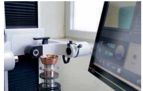
Non-contact measurement of grinding wheels in transmitted light on ZOLLER presetting and measuring machine
