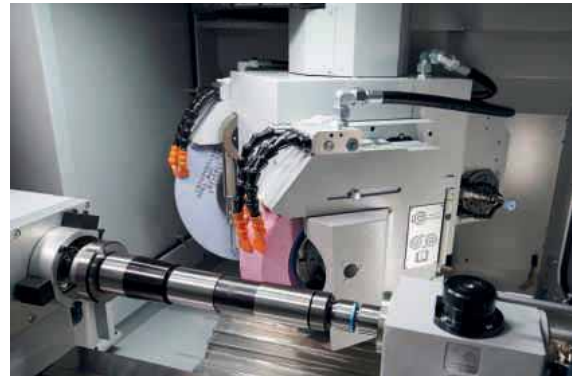
As featured the K10 can be fitted with a second external grinding wheel
