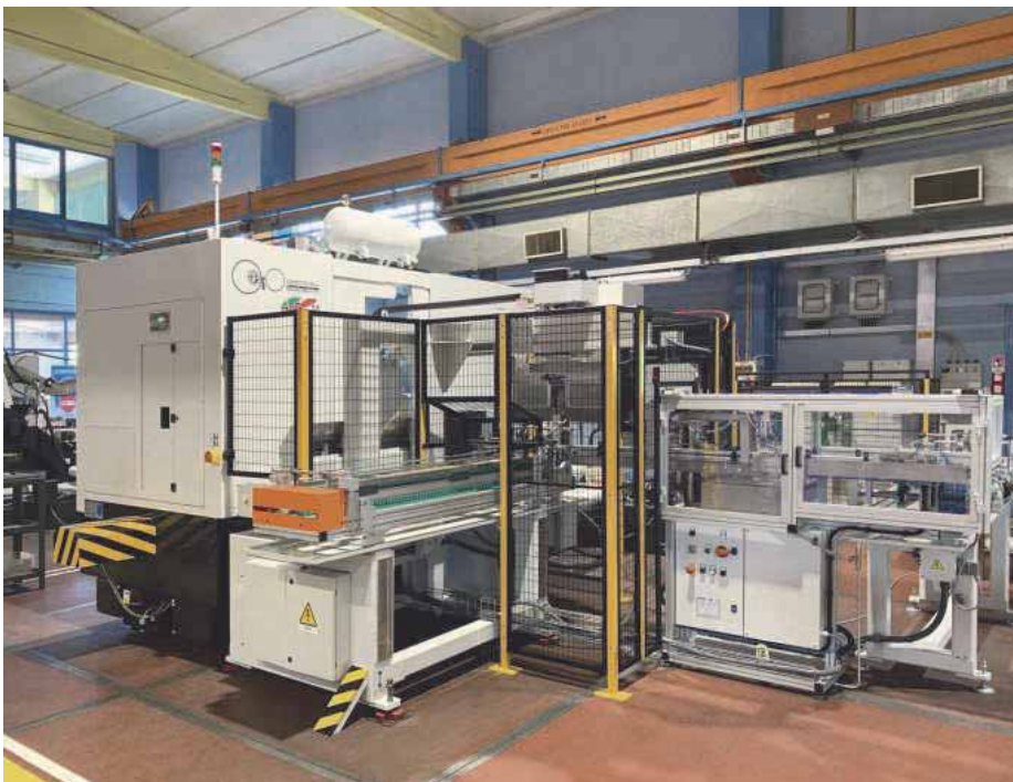
The APG-M machine lends itself to integrate subsystems such as loaders and post-process measuring stations
