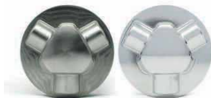
cnc inox socket joint before and after the finishing process
