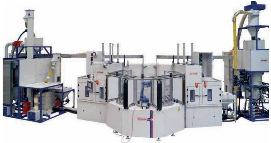
Large automated, robot loaded, twin blast machines, for shot peening turbomachinery turbine blades or medical implants
