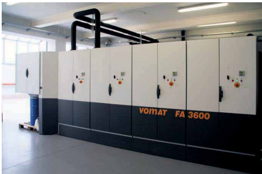
The central filtration systems from VOMAT consist of separate modules that can be scaled up in steps of 1,200 litres
