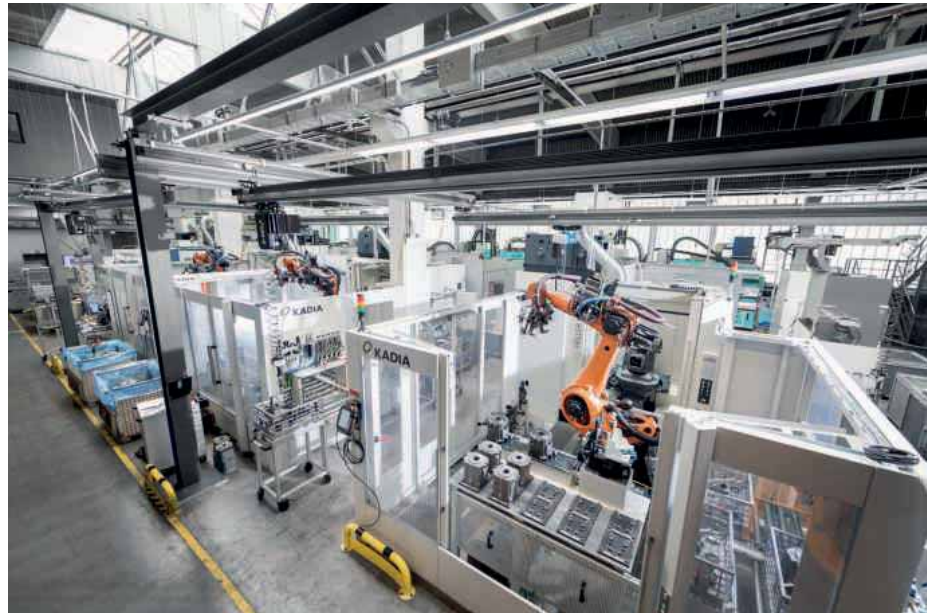
General view of the RHDC from KADIA and machining centre at ZSO. The two plant sections form a complete production unit and work closely together thanks to the interface and well thought out process design
