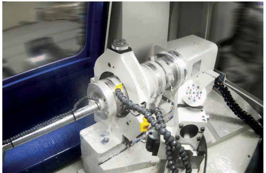
The GSB machine is designed for internal grinding process, face grinding and taper grinding
