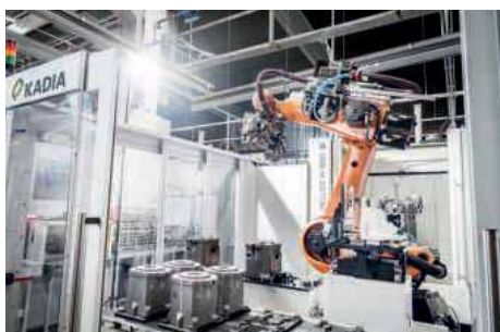
A view into the Deburr-Automation-Cell from KADIA. The cast iron housings are on pallets and are machined in the machining centre in a double pack
