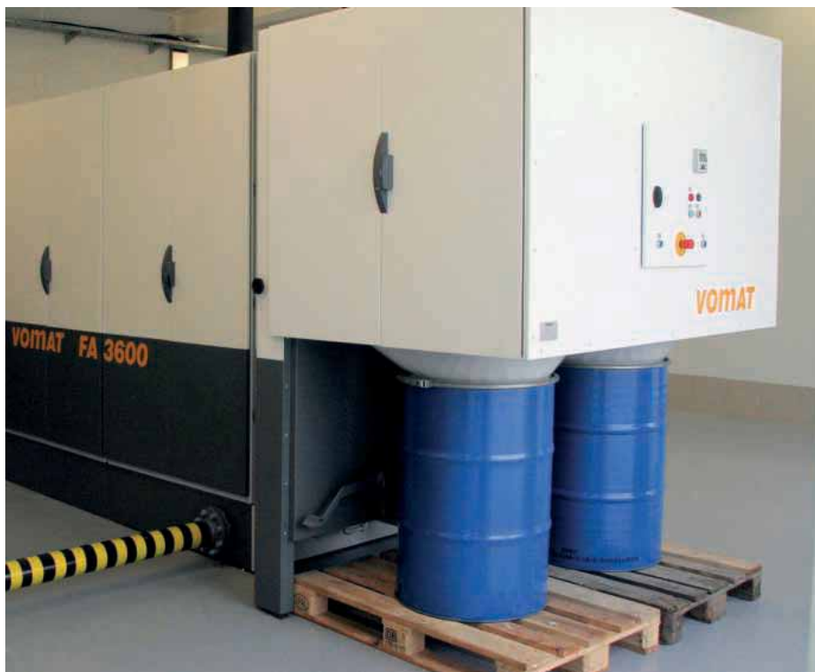
The recyclables are disposed of fully automatically directly into the transport containers provided by the recycling companies
